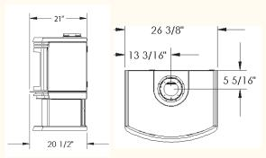
NOTE: When installing the Torino rear vent, a minimum 36" snorkel must be used. For detailed installation instructions, please refer to the Owners & Operators Manual.
